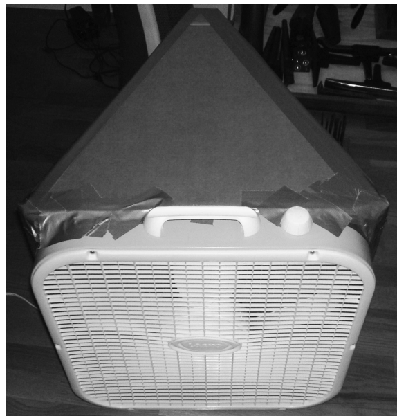
DIY HEPA filter for diesel particulate and woodsmoke
